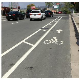
Figure 43 - Buffered Class II Bike Lane on Broadway -Oakland, CA.
