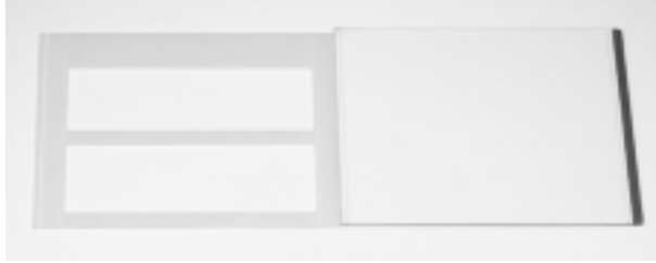
Fig 24. An opened Ettan DALT Precast Gel Cassette showing plastic frame cover (left) and glass plate (right).
