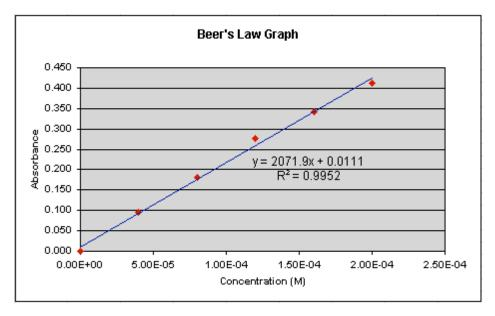
Figure 1. Calibration curve for yeast concentration as a function of absorbance measured at 520 nm.
