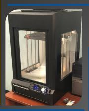
MakerBot's 3D Printers uses FDM technology to extrude, which acts similar to a hot glue gun. Plastic filament is fed in through the top, is melted at 215°C, and is "extruded" out of the nozzle into the layers that build a 3D print
