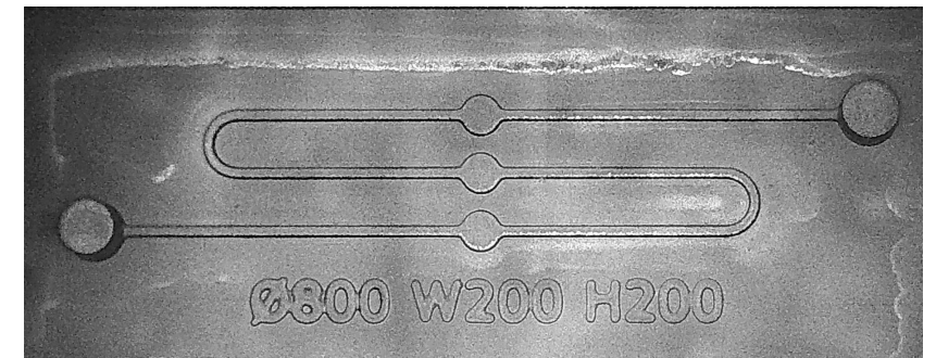
Microscope image of 200 \mu\text{m} wide microchannel with three \text{\O} 800 inline diaphragms,
