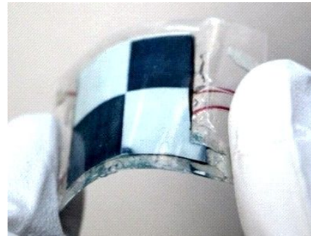
Four-pixel demonstration prototype for low-power "electronic paper" display.
