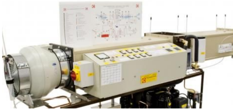
Commercial air conditioning lab unit
