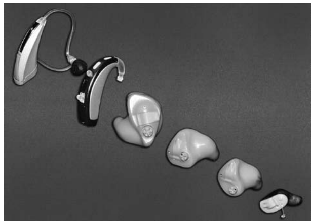
Figure 25. A family of hearing aids including the behind-the-ear style through the completely-in-the-ear style.
