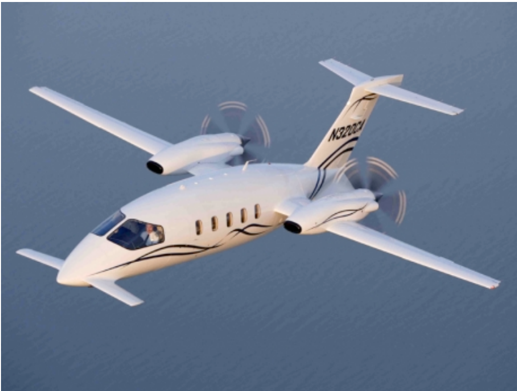
Figure 2.2 – The wing of the Piaggio P-180 Avanti may be approximated as a flat plate to illustrate a simple application of boundary layer theory in the estimation of skin friction drag.
