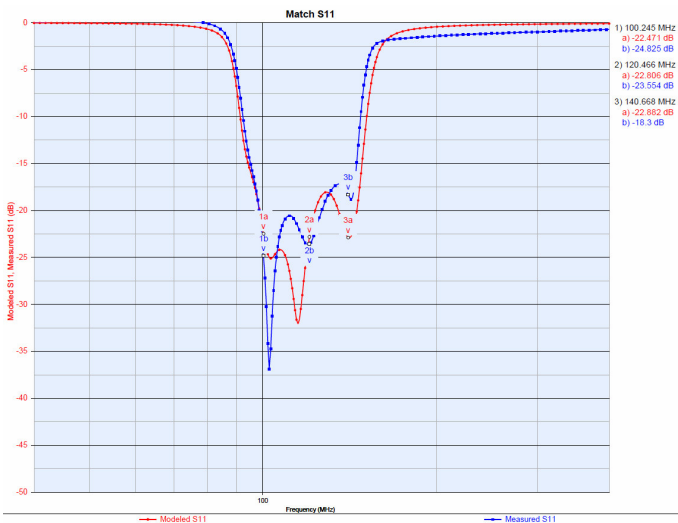
Figure (18) Simulated (Red) Vs. Measured (Blue) S11 Plots
