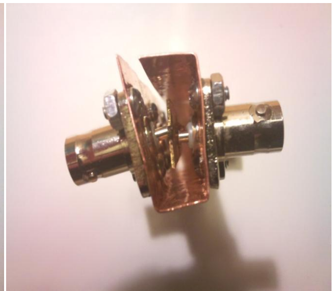
Figure 16. Side View of the Power Divider
