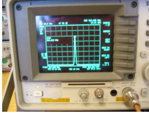
Figure 3.2. Transmitter output, centered at 915.2 MHz.
