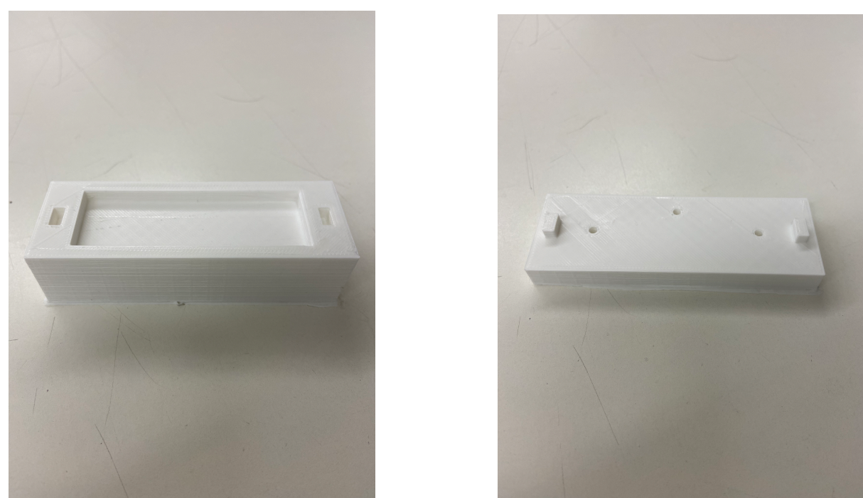
Figure 2: 3-D print of top and bottom part of flow chamber unit, printed in polylactic acid.
